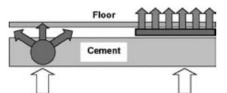
Standard underfloor heating is achieved with a cable or pipe embedded in the concrete screed. This means that a large percentage of the heat generated is actually absorbed in the concrete which in turn means higher consumption to achieve the desired heat.
