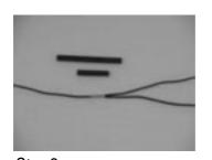
Step 2 Connect 4 mm crimp sleeve on the cable.
